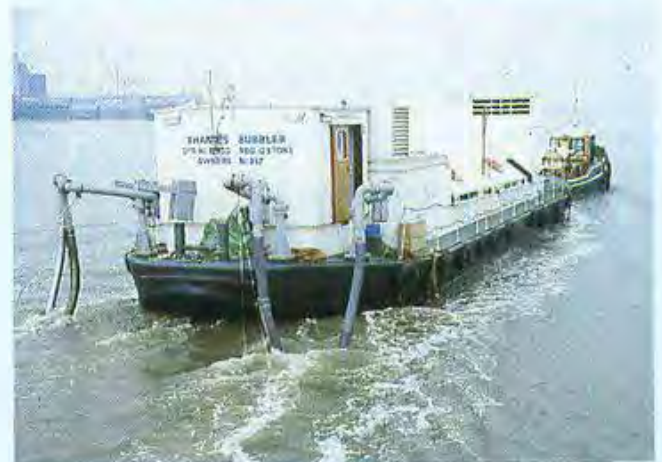
Fig. 3 The Thames Bubbler. Heavy storms sometimes wash extra sewage effluent into the river. The bubbler injects oxygen into the water to stop the oxygen level falling to a point where fish would suffocate.
