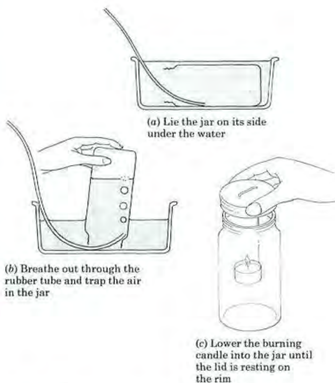
Fig. 13 Testing exhaled air for oxygen
